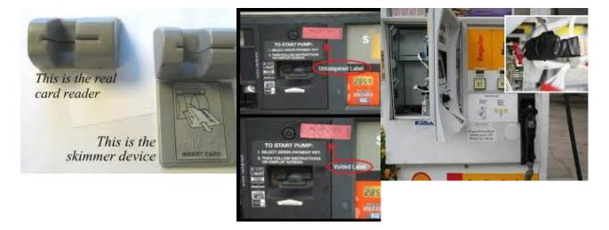
Security labels can help uncover skimming crime, in which a device is installed in the pump to steal data as payment cards are swiped through the reader.
